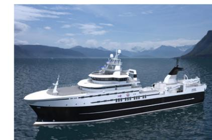
**NB1102** – An **85 meters** long Arctic Freezer Stern Trawler for an undisclosed reputable fishing company from **Faroe Islands**. The vessel will be an advanced, technologically sophisticated factory trawler capable for triple trawling. She will be outfitted with a shrimp factory, an advanced fillet factory and a fishmeal and fish oil plant. In addition there will be arrangement for freezing of pelagic species onboard the vessel.
