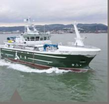
We delivered the first vessel of 2022 to Stromness Bay Limited. Being the first delivery of the year, the Longliner Factory Fishing Vessel "Polar Bay" has 60,5 meters overall length with 13,0 meters beam and she is powered by a 1920 kW Yanmar main engine.
