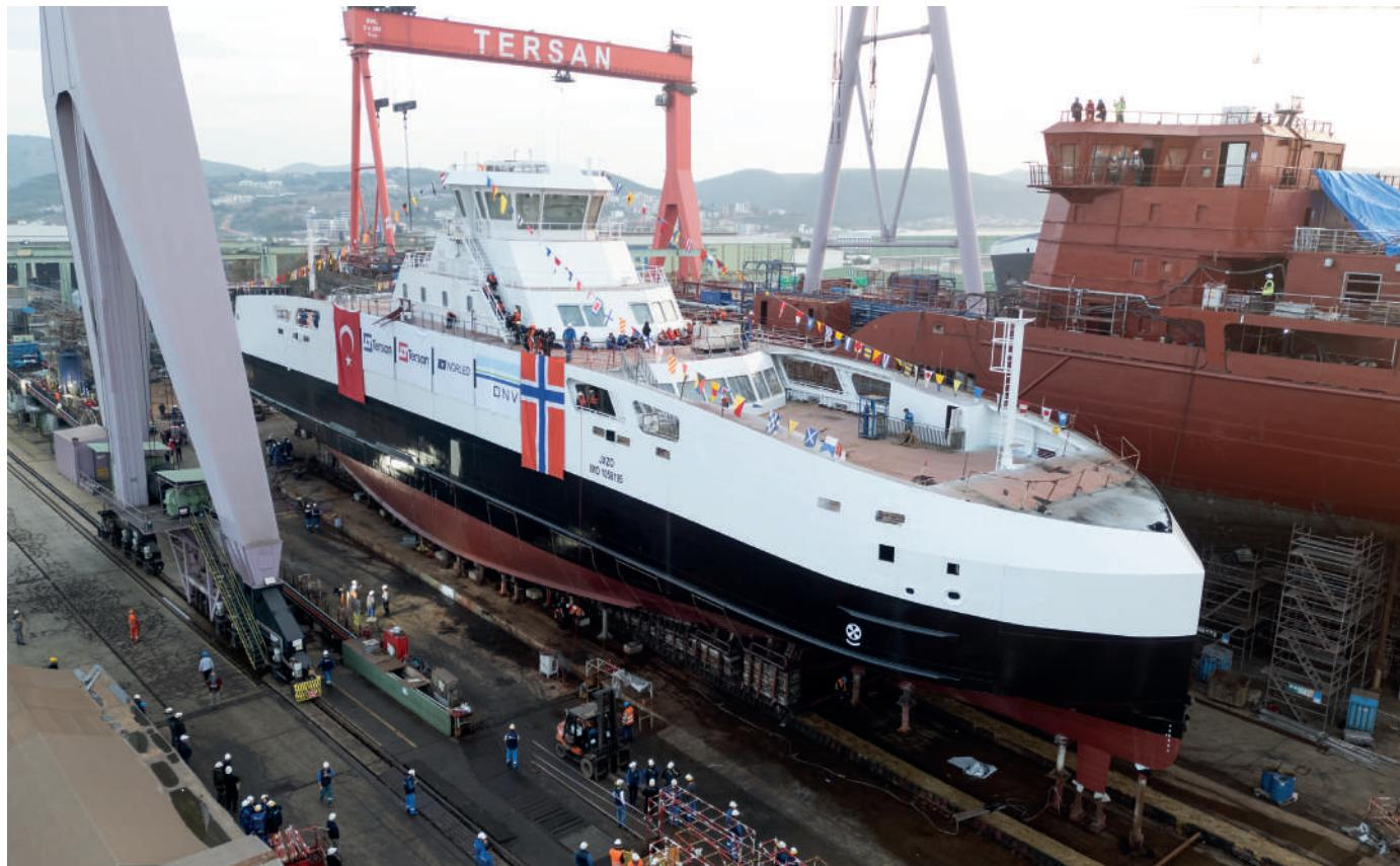
Measuring approximately 84.5 meters in length and 15 meters in width, the ferry will serve Norway's coastal routes with a capacity of 60 cars and 250 passengers. Equipped with a fully battery-supported hybrid system, the vessel contributes to low-emission maritime transport and supports Norled's sustainability ambitions.
