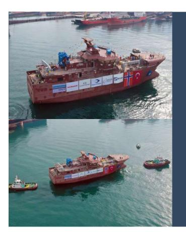
The vessel having a 60.5 meters overall length with a 13,0 meters beam will be powered by Yanmar 6EY26W main engine and she will have comfortable accommodation up to 30 people on board. She will be the 6th vessel to be built for Ervik Havfiske while the first 5 vessels including Froyanes Junior and Vestkapp which are delivered last year, are successfully conducting fishery operations.
