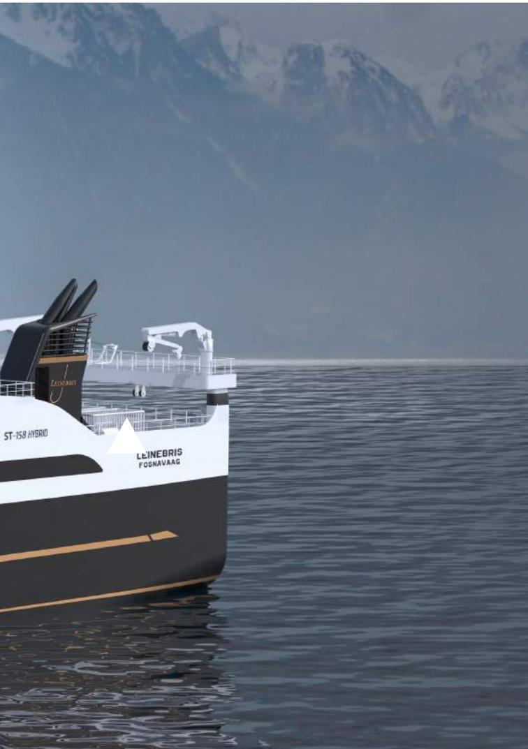
64.9 meters long and 15 meters wide Leinebris will ensure the safety of the crew with double cargo decks, covered working decks and the moonpool. She will also have RSW tanks to be able to catch fish alive for fresh production or for the possibility to unload directly from the tanks to shore.
