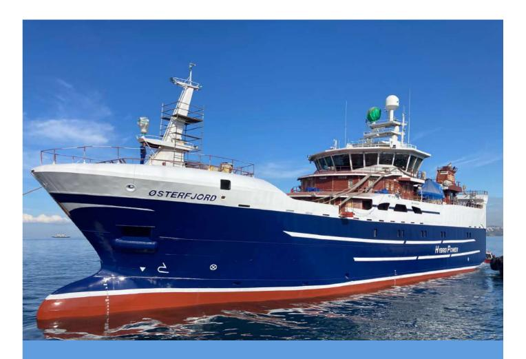
NB1098; Longliner Factory Fishing vessel which to be named as ØSTERFJORD will be also delivered by the mid. of last quarter. She is an advanced vessel with different types of fishing methods, like longlining,
